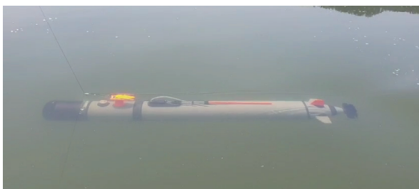
AUV under development: way point tracking test
