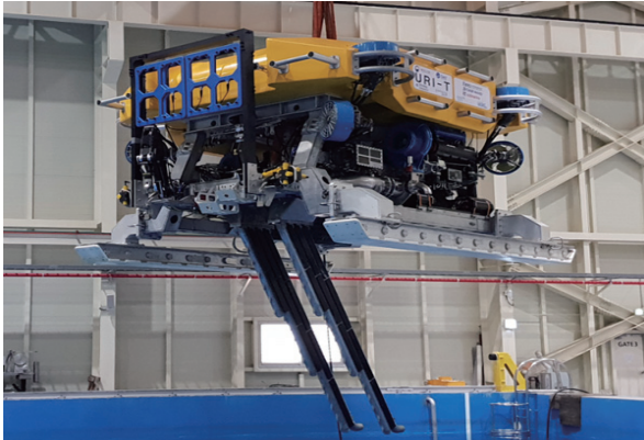
URI-T, an underwater cable burying ROV
